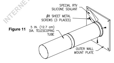
9. From outside the building, slide the five (5) inch (12.7 cm) diameter telescopic tube through the opening in the wall until the outer wall mount plate is flush with the wall (See Figure 12).
